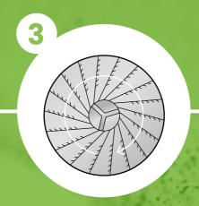
Emulsion hits the rotor cap of the rotating tool and is evenly
