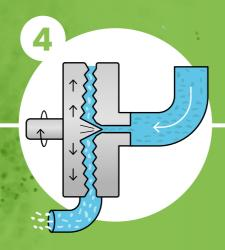
Flakes are aligned parallel to tools in the infeed zone. Gap (0-30 mm)
