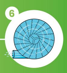
Flakes move outward in a spiral over tools and are cleaned several times in the process.
