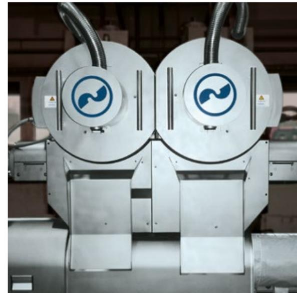
**Screen changes without stopping the machine** – for continuous production: this special execution of the EREMA Laserfilter LF 2/354 TWIN makes it possible
