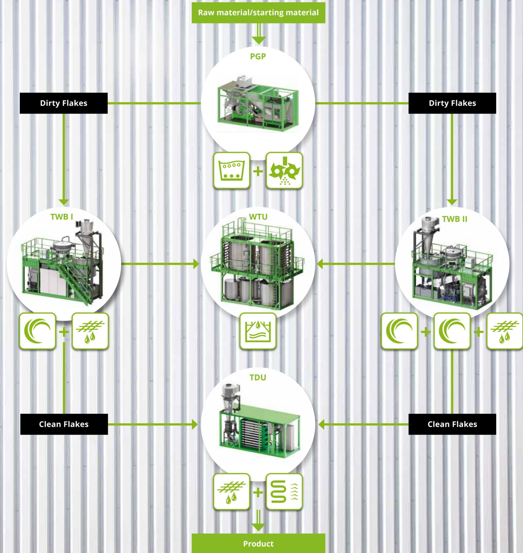
Solo and as a team: Each container covers one work step in the process. The HydroDyn® UCC system is thus equally suitable for installation in new industrial washing plants as for installation as part of retrofitting existing plants to improve process quality and cleaning efficiency.
